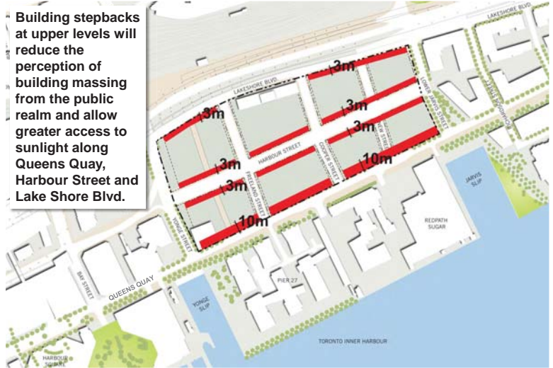
Stepbacks: Queen's Quay, Harbour Street and Lake Shore Blvd (stepbacks not to scale)
