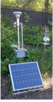
Photo of Typical Air Monitoring Station
