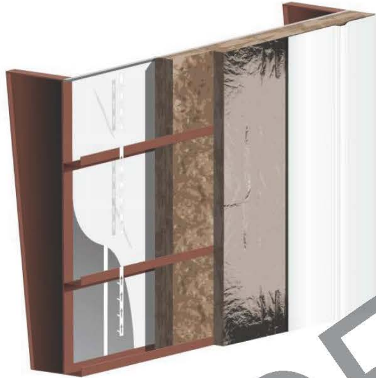
Figure 6: Energy Saver Wall System with Primary Insulation Layer between Girts and Secondary over Girts
