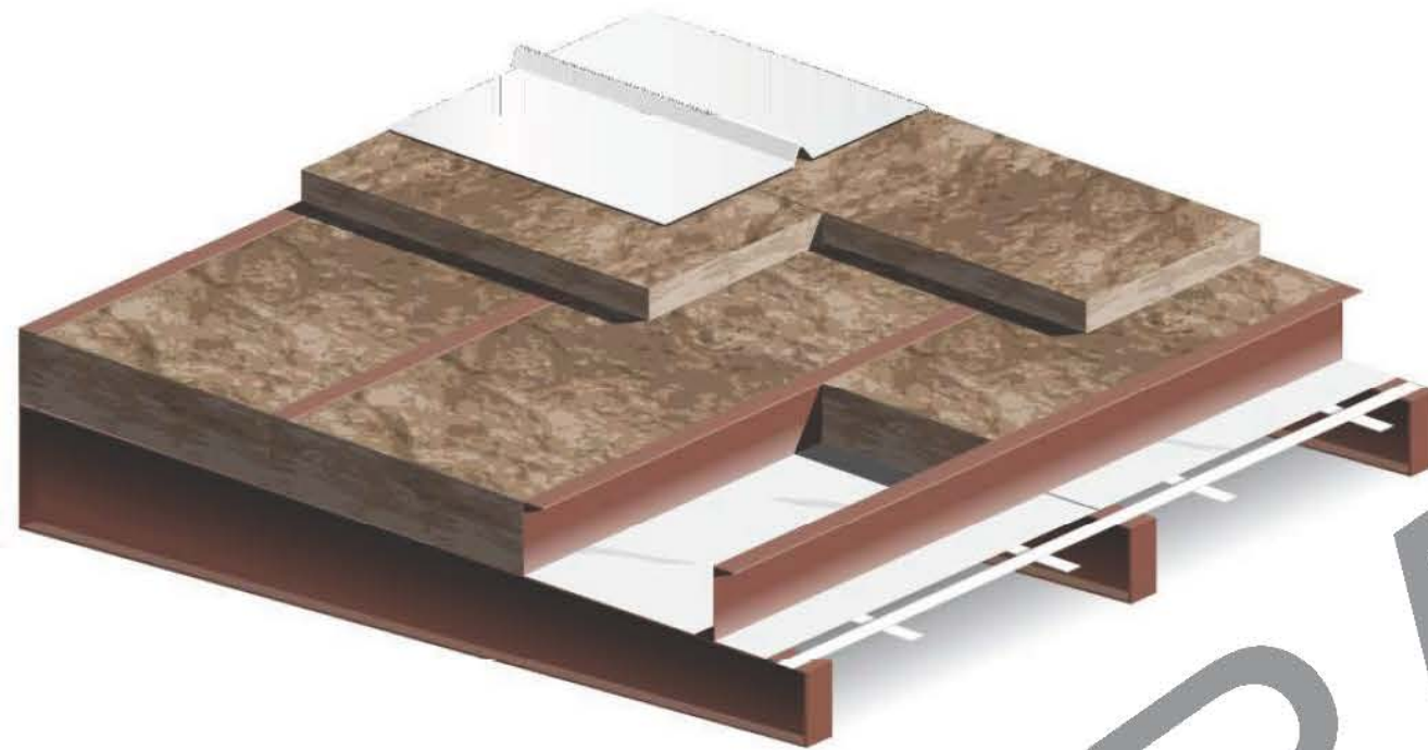
Figure 3: Energy Saver Roof System with Primary Insulation Layer between Purlins and Secondary above Purlins
