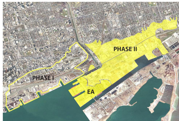
Figure 2 DMNP EA Flood Plain Map Illustrating the areas that are currently at risk of flooding under the Regulatory Flood Event
