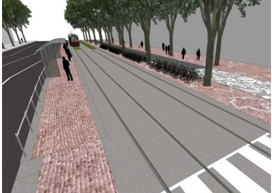
Bicycle racks perpendicular to tracks
