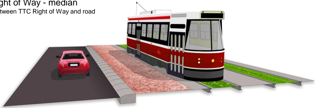
Grey granite curb stone 250x600x1000mm
